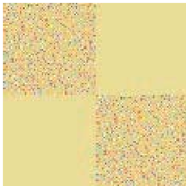
Fig. 10. Influence of radiometric attributes and spatial considerations on visual "homogeneity": observers will see four squares even if the two textured ones have a very important radiometric inhomogeneity.
