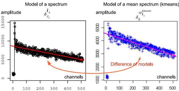
Fig. 16. *Minimisation of the  $L_1$  distance between the model of the mean spectra  $\delta_k^{sp_{\hat{\mathbf{f}}_\lambda}^{kmeans}}$  and the model of the spectra at each pixel  $\hat{\delta}_{x_i}^{\hat{\mathbf{f}}_\lambda}$ .*
