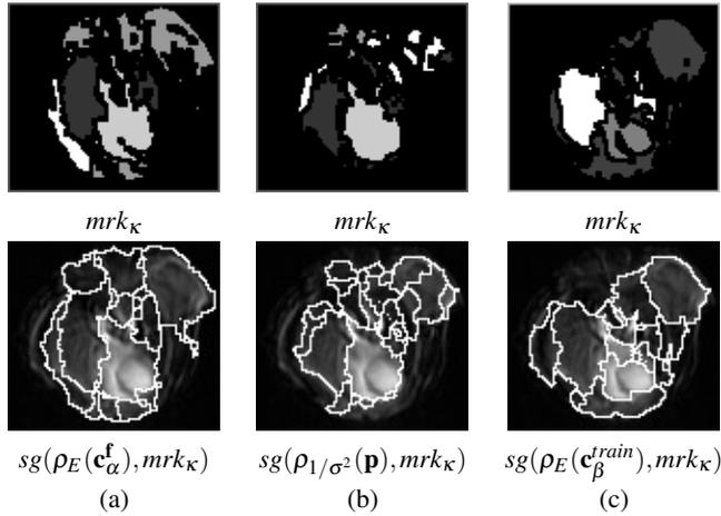
Fig. 28. Segmentations by marker-controlled WS into several spaces: (a) in the factorial space  $\mathbf{c}_\alpha^f$ , (b) in the parameters space  $\mathbf{p}$  and (c) in the PCA space of the training set on the parameters  $\mathbf{c}_\beta^{\text{train}}$ . The gradient-based distances are the same as in Fig. 27. The markers come from the LDA classification for the different image spaces.
