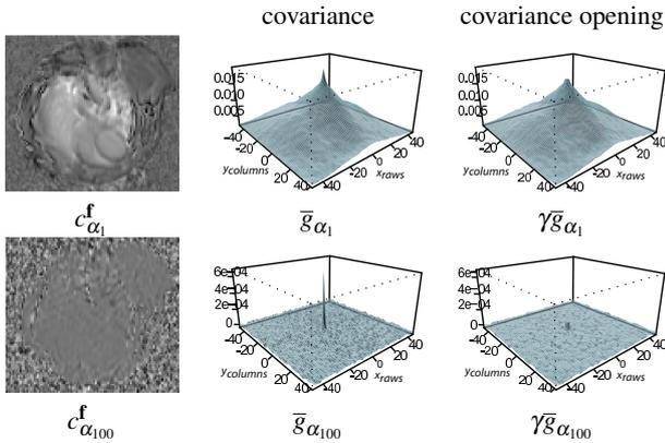
Fig. 7. Covariance before ( $\bar{g}$ ) and after a morphological opening ( $\gamma \bar{g}$ ) on the factor pixels channels  $c_{\alpha_1}^f$  (without much noise) and  $c_{\alpha_{100}}^f$  (noisy channel).
