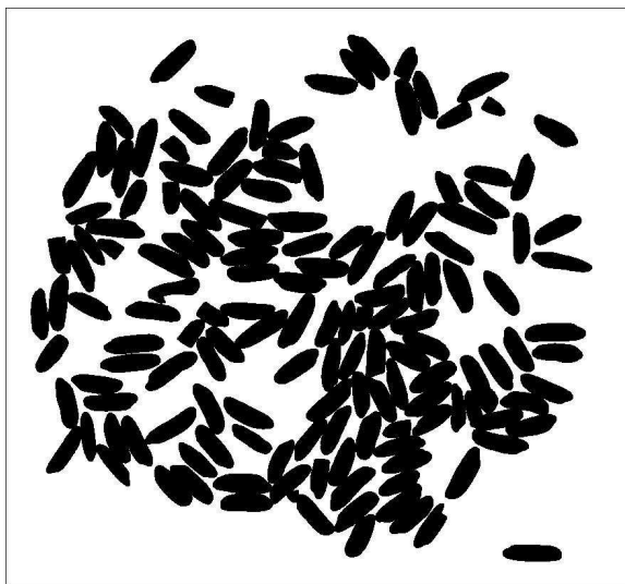
Fig. 6. Binary image obtained with the Otsu algorithm applied on the grey-level image (Fig. 4).
